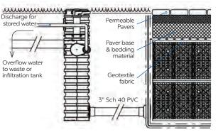
Vaults can be located adjacent to the reservoir or remotely. For remote installations use dual 3" pipes between the Pump Vault and the reservoir. Flow capacity decreases as the distance between the vault and reservoir increases.
