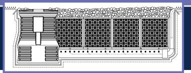
Atlantic's Eco-Blox and Pump Vaults make excellent, easy to maintain bog filters. With a perforated pipe under Eco-Blox, the Pump Vault acts as a cleanout for upflow bogs of any size. Pond water pumped into the bottom of the Eco-Blox reservoir sheds velocity which causes sediment to settle out. Plants set in a thin layer of gravel on top of the Eco-Blox remove fine solids and nitrates. Simply flush the chamber from above into the Pump Vault to remove sediment.
