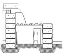
SPILLWAY WITH FORMAL SPILLWAY BASIN
